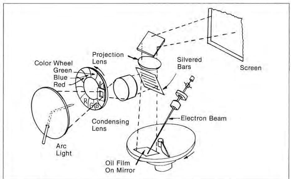
**Fig. 1:** The first television light valve was the Eidophor, invented by F. Fischer of the Swiss Federal Institute of Technology.
