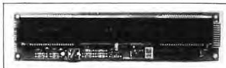
The Industrial Products Division of IEE has added a new low-cost 5 x 7 dot-matrix 1 x 40 display to its FLIP™ line of intelligent vacuum fluorescent display modules. Designated as model 3601-84-040, this no-frills module is suited for high-volume OEM applications, such as copiers, point-of-sale terminals, and security systems. It displays a full 40-character line, yet is extremely compact, measuring only 9.45" (W) x 2.20" (H) x 0.77" (D). Characters are 0.2" (5.1 mm) high.
