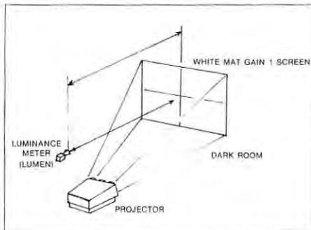
Fig. 1: Measurement of brightness.
