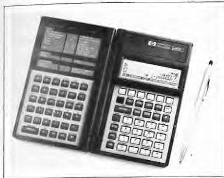
Hewlett-Packard Company has introduced the HP-28C technical professional calculator, believed by its manufacturer to be the first calculator capable of performing symbolic mathematics.
