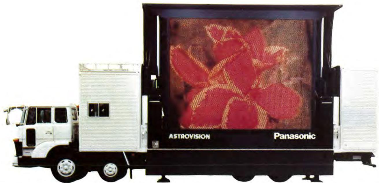
**Fig. 4:** Matrix displays, such as Panasonic's portable Astrovision, are currently the only displays bright enough for use in direct sunlight, but their resolution is not as good as that of light-valve projectors.
