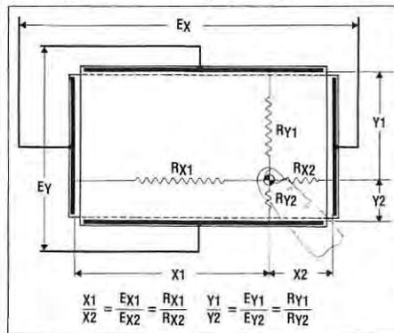
3]. Alternatively, each can have opposing bus bars which are orthogonal to those on the other element to create linear potentiometers in the X and Y axes. When a voltage is impressed on each element alternately, the voltage division at the contact point, as sensed by the other element, produces X and Y voltages that are analogous to the X and Y contact positions. An analog-to-digital converter then translates the signal to computer-readable form. This is the "analog panel" approach [Fig. 4].
