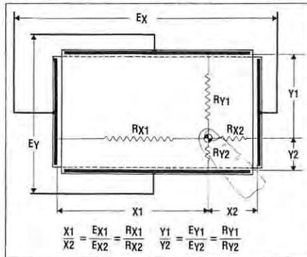
3]. Alternatively, each can have opposing bus bars which are orthogonal to those on the other element to create linear potentiometers in the X and Y axes. When a voltage is impressed on each element alternately, the voltage division at the contact point, as sensed by the other element, produces X and Y voltages that are analogous to the X and Y contact positions. An analog-to-digital converter then translates the signal to computer-readable form. This is the "analog panel" approach [Fig. 4].
