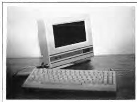
A light-emitting flat-panel terminal from Emerald Computers, Inc. combines previously unutilized flat-panel benefits and conventional system access technology. The device has been designed to provide multiterminal users with a light, durable, compact alternative to conventional CRT terminals, without the disadvantages of electromagnetic distortion, mechanical vulnerability, eye strain, and ambient radiation.
